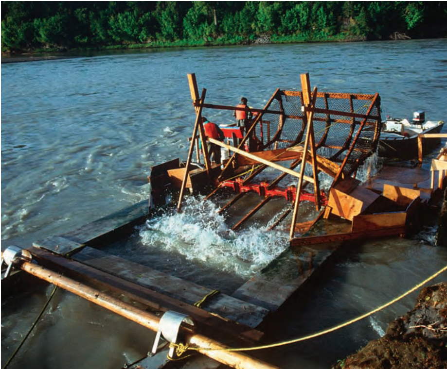
Figure 3.33 The Nisga'a First Nation in the Nass Valley produces aluminum fish wheels that are based on a traditional wooden design. The Nisga'a use the fish wheels to catch salmon swimming upstream, enabling them to count, weigh, and measure them.
