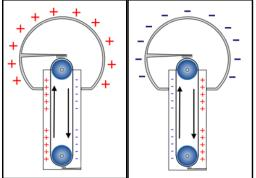
**Van de Graff generators** (VDG) use friction to produce a large amount of static charge (see page 253)
